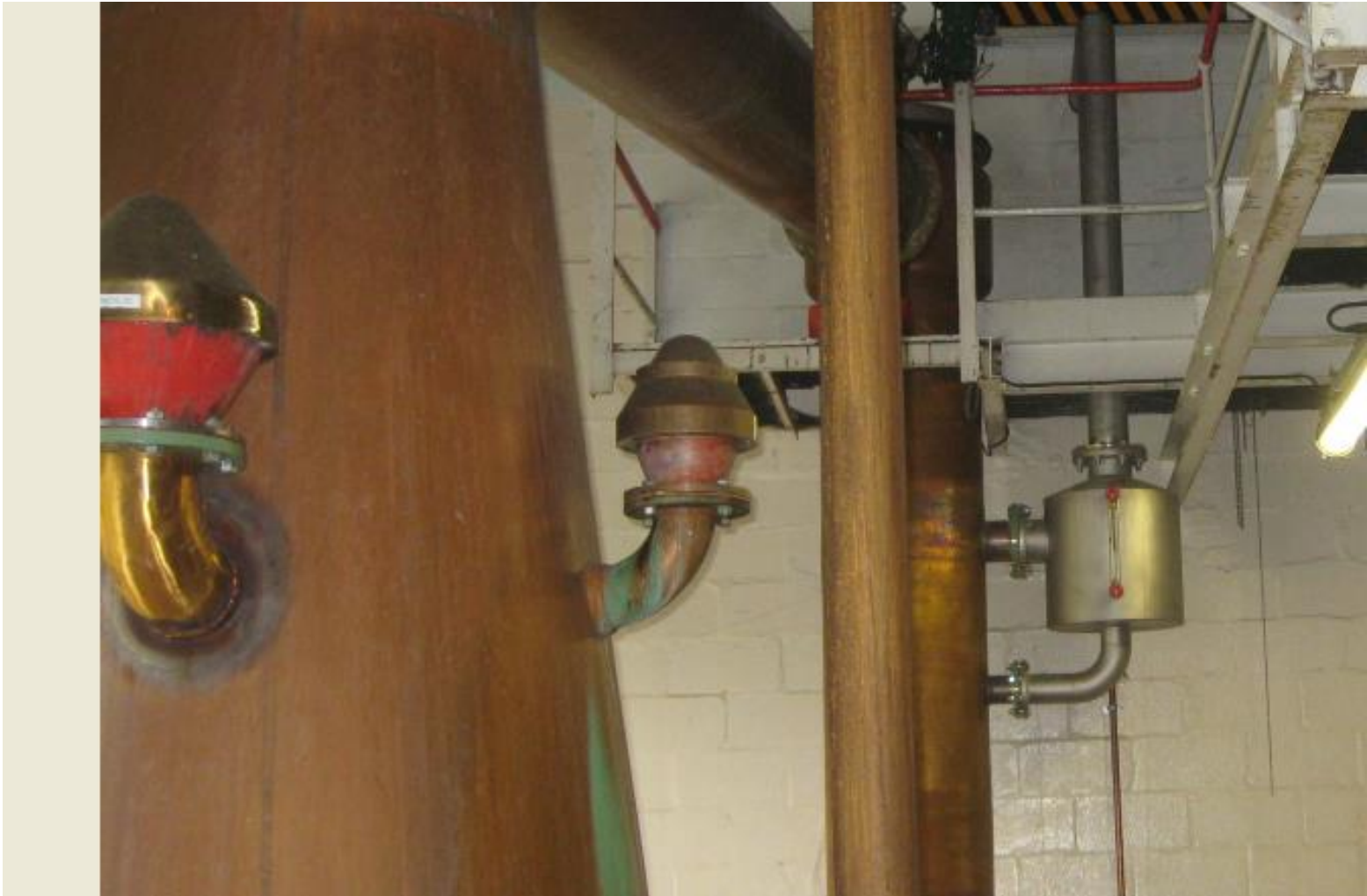
Example - Bubble Pot and Anti Vac Valves On a Pot Still
