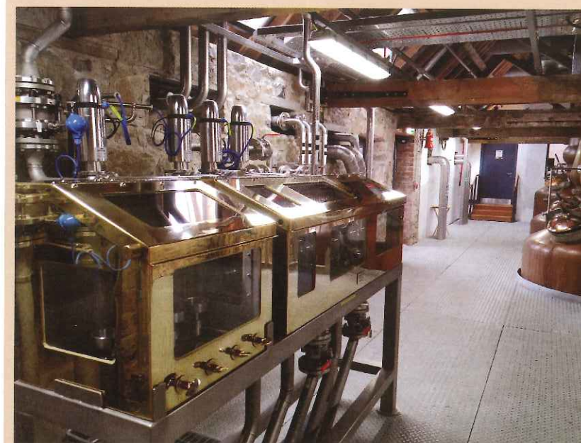
Traditional spirit safes, but with ultra-modern valving behind the system
