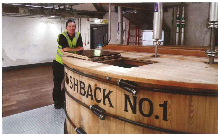
Enda Rice, maintenance manager, at one of the 30,000 litre washbacks. Given current production volumes the vessels are half-filled only, with a single brew of 13,200 litres
