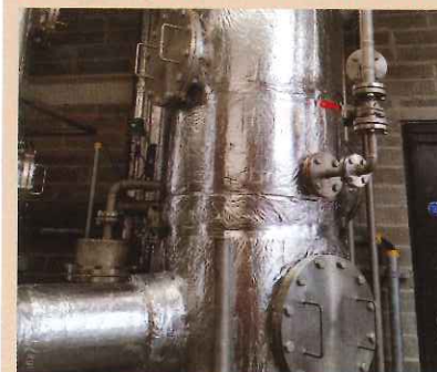
One of the McMillan column stills, made from copper but surrounded by insulation, and soon to be clad in sheet metal
