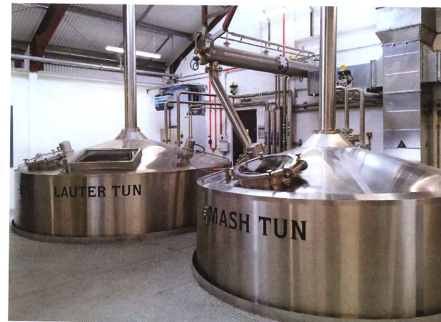
Interior of the distillery buildings housing the mash house. A Steele's masher supplies milled grain to either the lauter tun directly or to the mash tun
