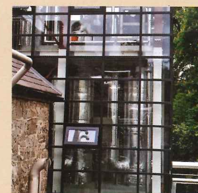
An external view of the column still house with condensers on top
