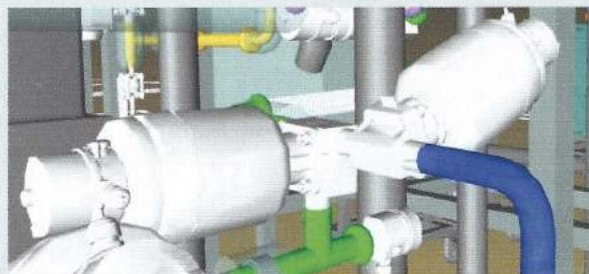
'T' DIAPHRAGM VALVE (ALSO KNOWN AS ZERO DEAD LEG) AND 2-WAY DIAPHRAGM VALVE
